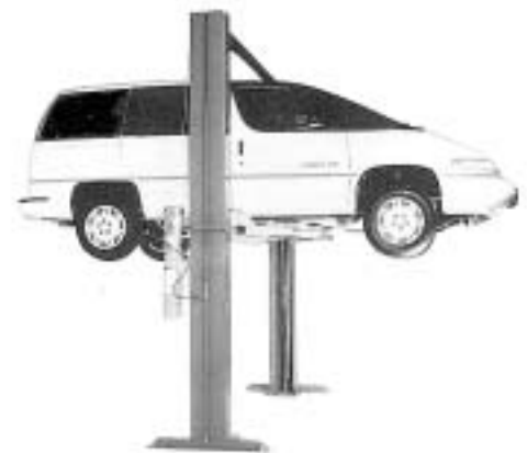
Narrow columns with small base and few anchor bolts provide minimal stability.
