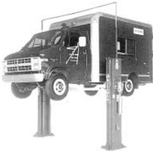
Mohawk's carriages (top) grip the arm distributing the load (↑) throughout vs. competitive lifts with 100 percent shearing force (↑) on the arm pin.
